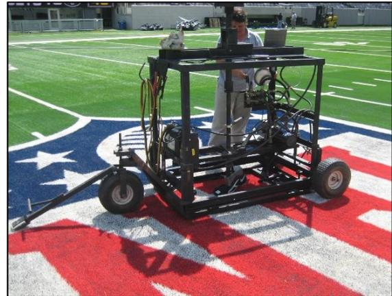
Figure 1. Pennfoot traction tester
