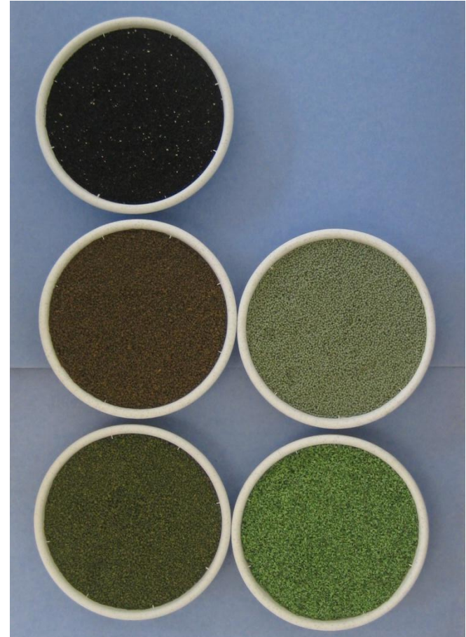
Figure 3. Various infills were tested including colored crumb rubber (left), EcoFill (bottom right), and TPE (middle right)
