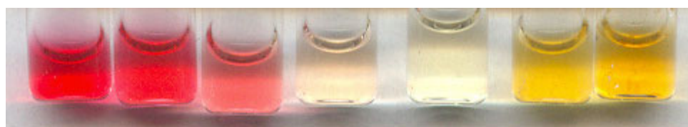
Figure 3-4. Demonstration of the effect of pH on anthocyanin color. Seed extracts were placed in different buffered solutions, pH 1-7, from left to right.
