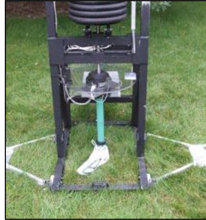
Figure 5. The traction tester used by researchers at Michigan State University (Villwock et al., 2009 a;b) tests rotational traction in a flat-footed stance and the weight distributed at the rear portion of the foot.
