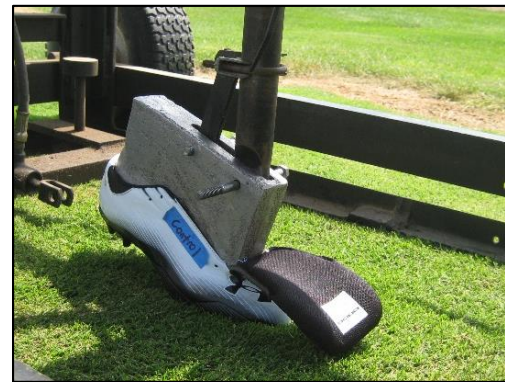
Figure 6. Pennfoot tests rotational traction in a forefoot stance with the weight distributed onto the forefoot as required by ASTM
