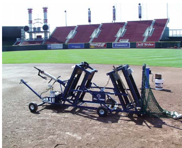
Figure 1: PENNBOUNCE measuring the pace of a skinned (grass-free) infield surface
