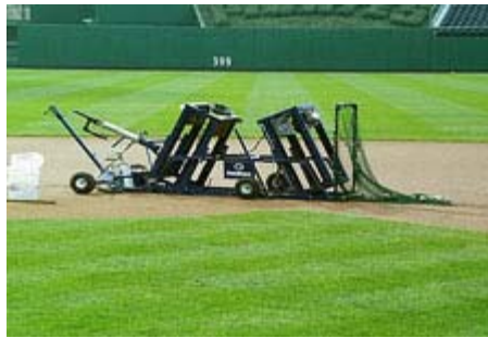
Fig. 1. Pennbounce apparatus for measuring playing surface pace (COR).
