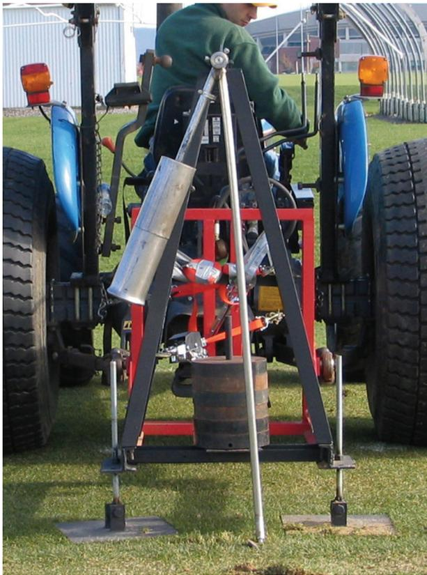
**Fig. 2** A weighted pendulum with a golf club head attached to one end that was used to create divots
