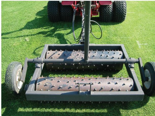
**Fig. 1** The Brinkman traffic simulator that was used to simulate athletic field use
