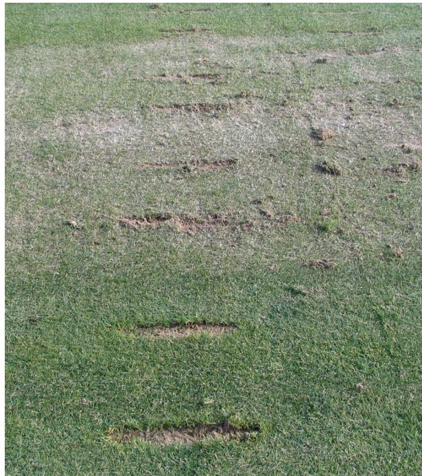
**Fig. 3** Divots created by the weighted-pendulum device
