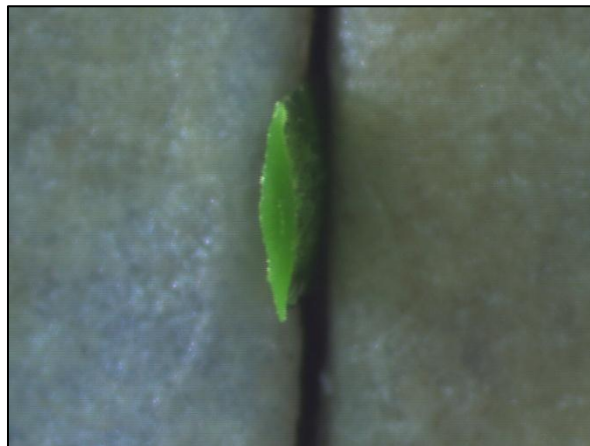
Cross section of Hellas Matrix fiber from sample tested.
