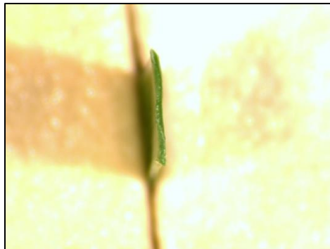
Cross section of Sprinturf Ultrablade DF monofilament fiber from sample tested.
