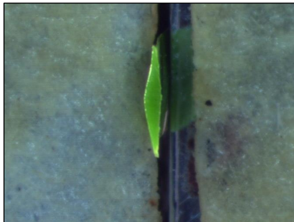
Cross section of Shaw Sportexe PowerBlade HP+ fiber from sample tested.
