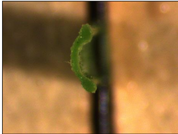
Cross section of AstroTurf GamedayGrass 3D with Astroflect fiber from sample tested.
