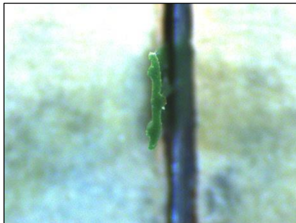
Cross section of Mondo Monofibre 3NX fiber from sample tested.
