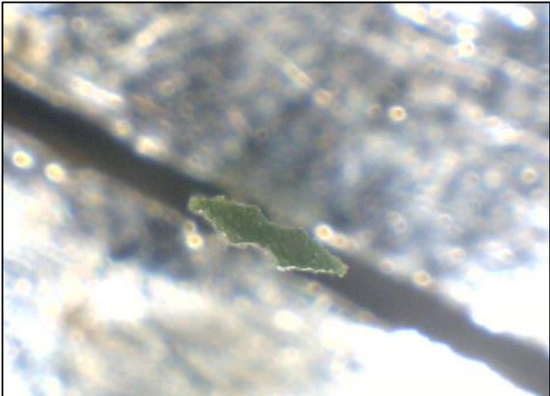
Cross section of FieldTurf Revolution 360 fiber from sample tested.
