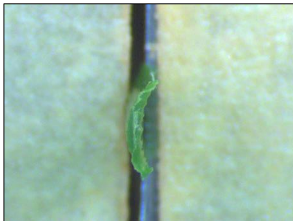
Cross section of FieldTurf Revolution fiber from sample tested.
