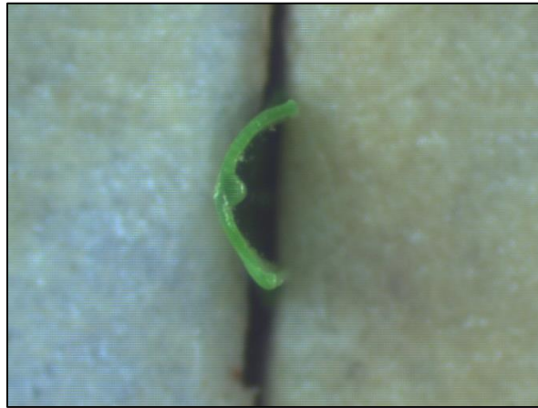
Cross section of FieldTurf Duraspine Pro fiber from sample tested.
