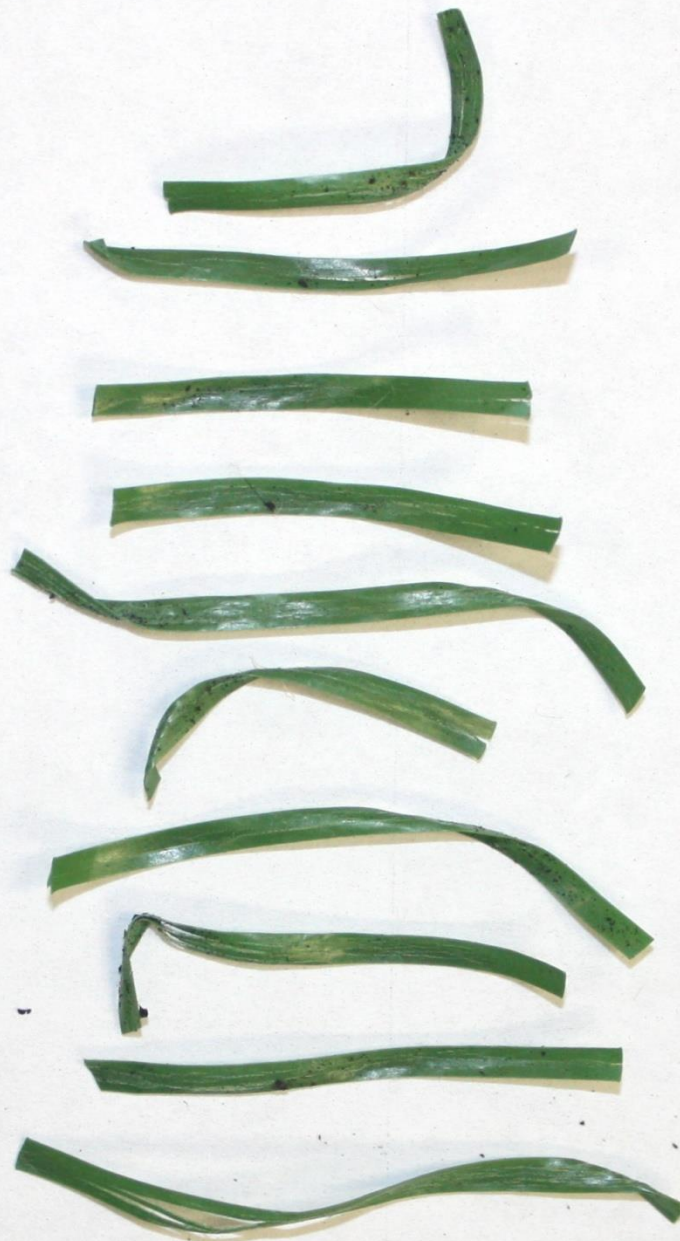
Sprinturf Ultrablade DF (monofilament fibers only) 20,000 Cycles
