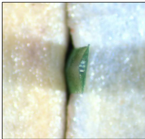
Cross section of UBU Sports Speed M6-M fiber from sample tested.
