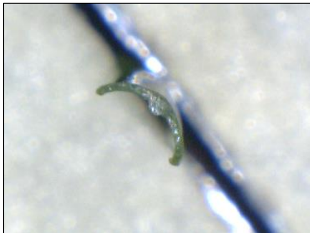
Cross section of GreenFields MX fiber from sample tested.
