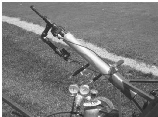
FIG. 2—Storm 300 Air Cannon used to propel baseballs.
