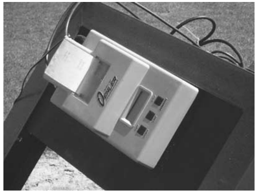
FIG. 5—Chronograph used to calculate velocity values.
