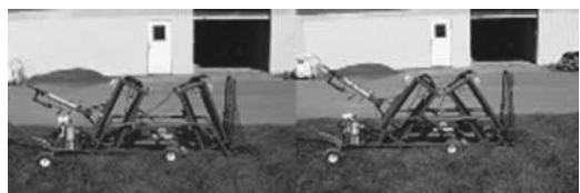
FIG. 7—Pennbounce configured to collect data in the 0.44 radian (left) and 0.61 radian (right) impact angle positions.
