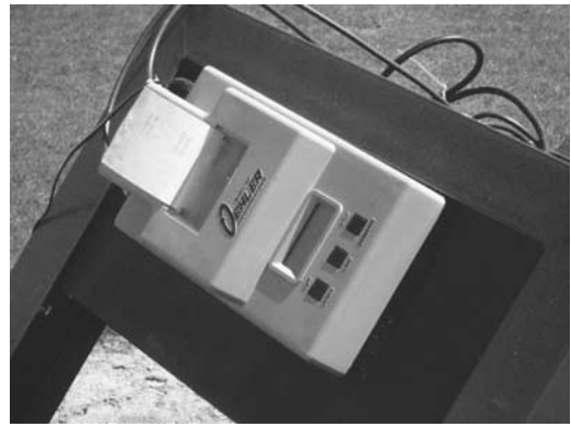
FIG. 5—Chronograph used to calculate velocity values.
