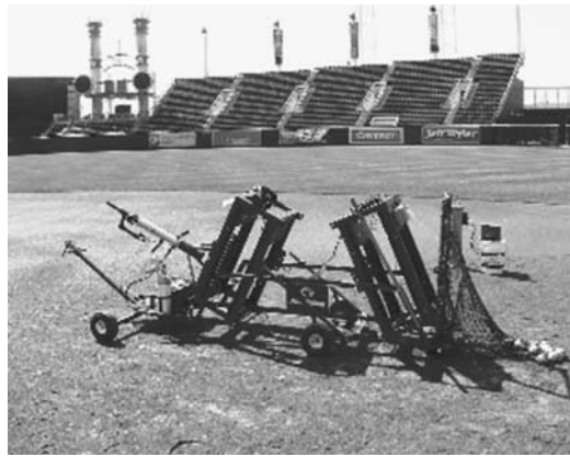
FIG. 1—Pennbounce apparatus for measuring playing surface pace.
