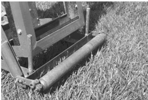
FIG. 9—Roller mounted to the rear of the frame.
