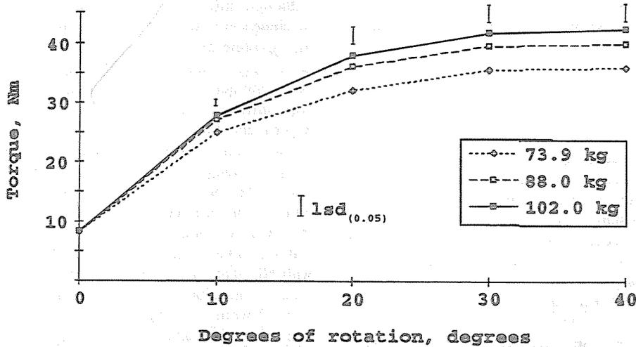
FIG. 7—Mean rotational traction forces for loading weights across grass species and cutting heights.
