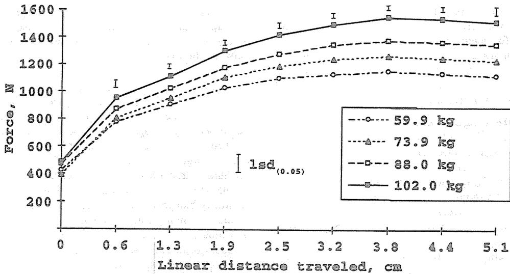
FIG. 6—Mean linear traction forces for loading weights across grass species and cutting heights.
