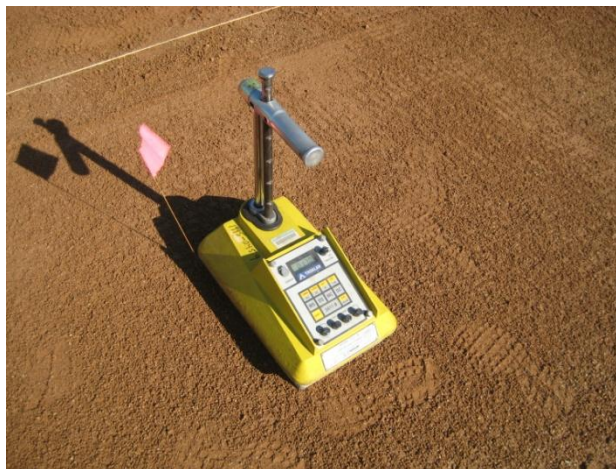
Figure 12. Troxler 3400-B Series moisture density gauge
