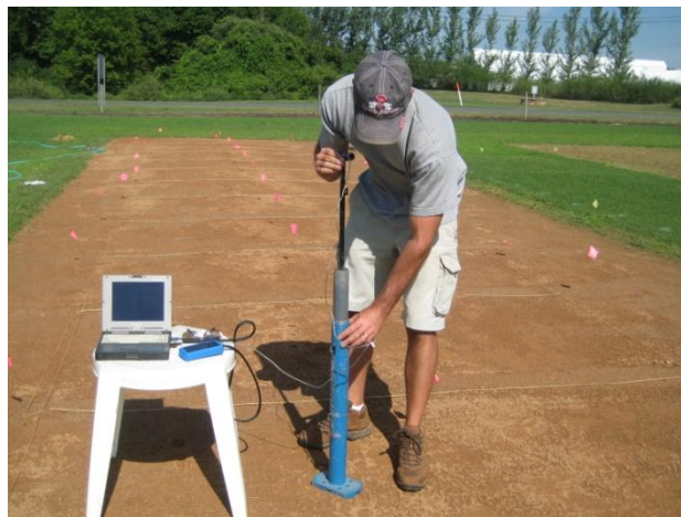
Figure 14. The Clegg Impact Tester was used to evaluate surface hardness
