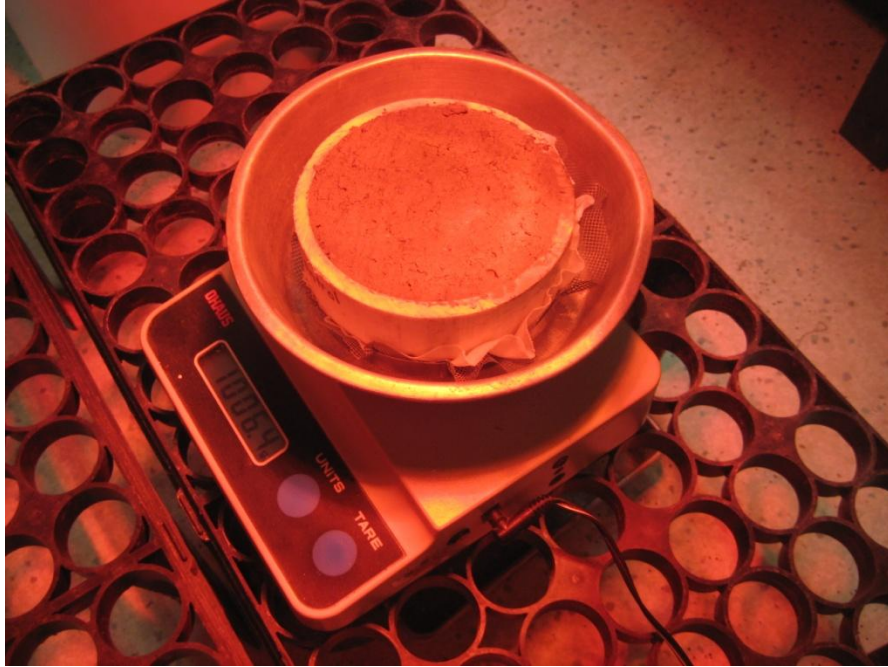
Figure 221. Each sample was placed onto a scale under a heat lamp
