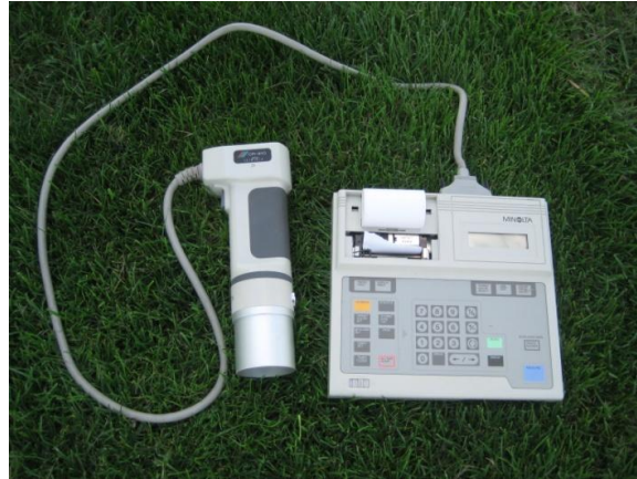
Figure 15. Chromameter used to measure surface color
