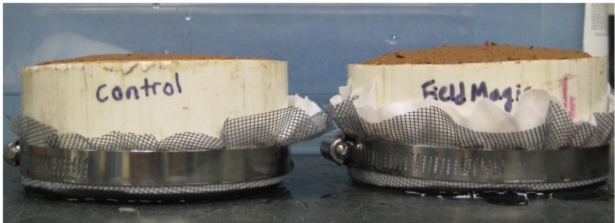
Figure 21. After saturation, the Field Magic sample increased in volume to a greater extent than the control
