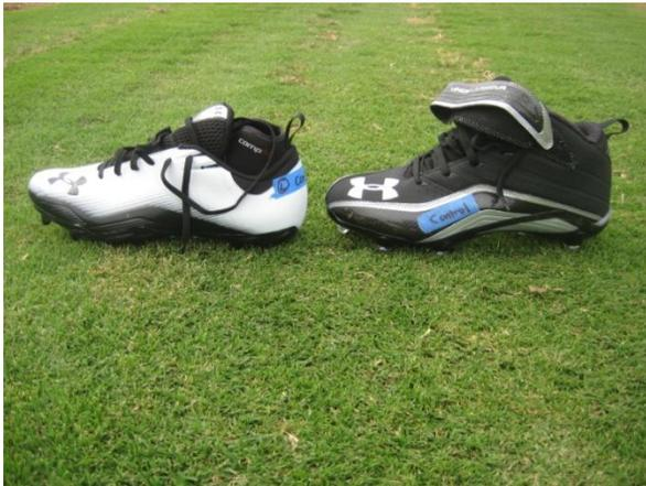
Figure 2. Testing was conducted using the Under Armour Nitro III Low CompFit shoe (molded) (left) and the Under Armour Fierce III D shoe (screw-in) (right)
