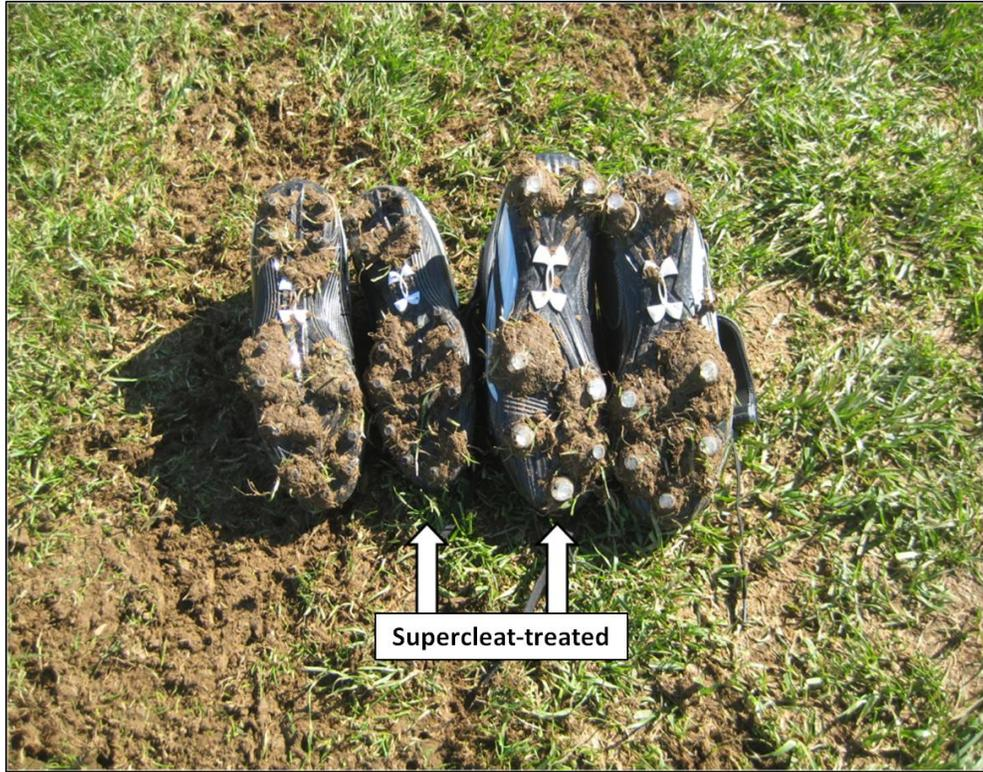
Figure 6. Soil accumulation at the second test location
