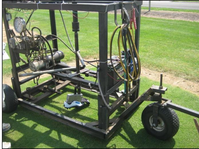
Figure 1. Pennfoot traction testing device
