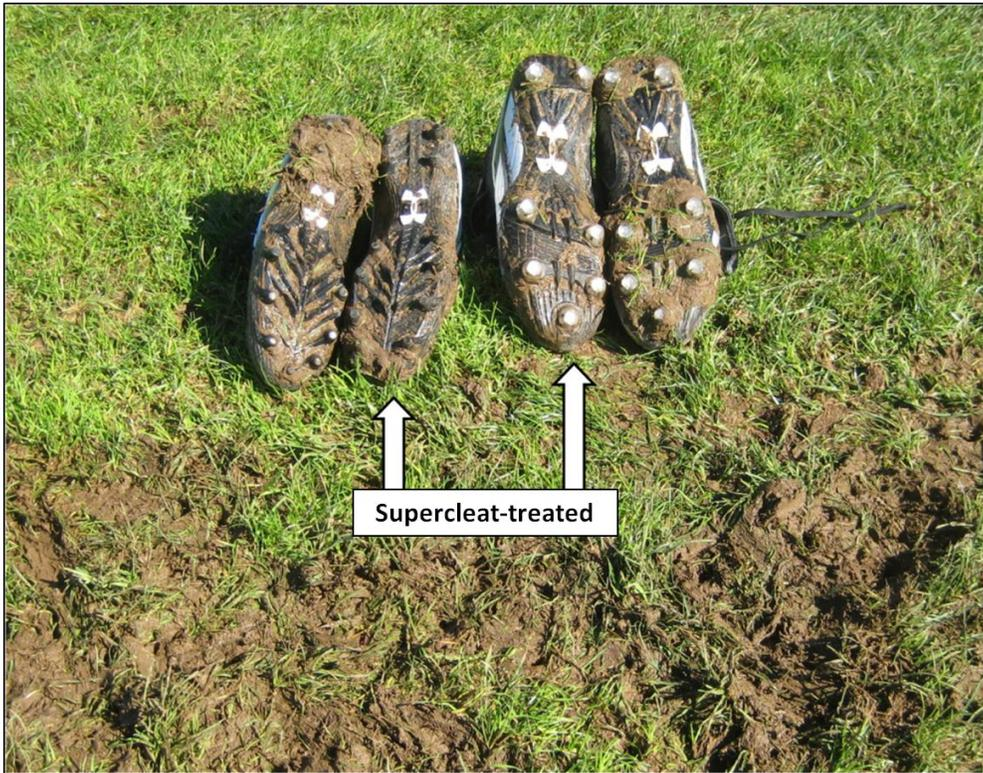
Figure 7. Soil accumulation at the third test location
