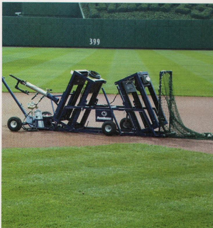
Pennbounce apparatus used to measure the speed of skinned infields.
