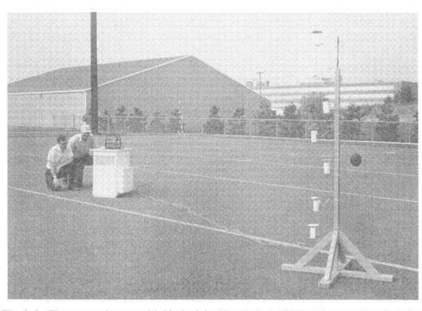
Fig. 3-2. Thermocouple trees with black globe placed on artificial turf. Instrument in center is pyroheliometer. (From Buskirk et al., 1971.)
