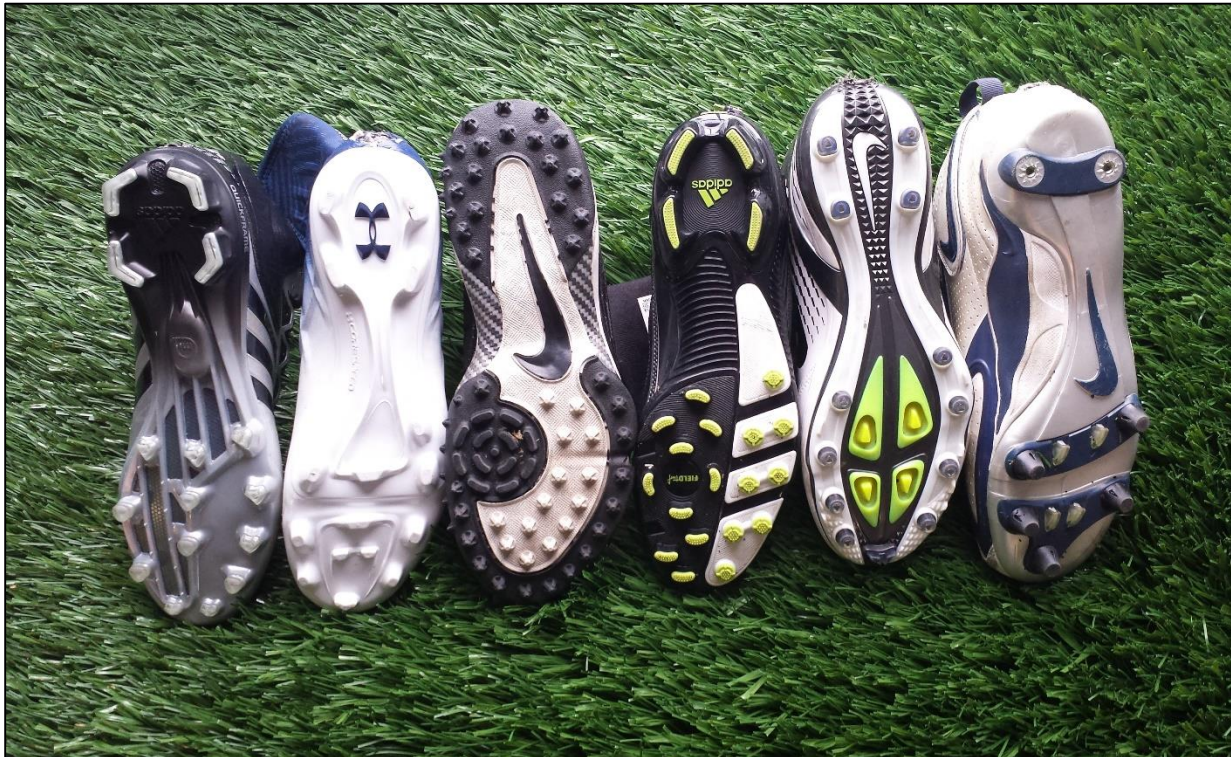
Figure 6. The shoes used in the traction testing were (from left to right) Adidas CrazyQuick Mid (hybrid), Under Armour Highlight MC (hybrid), Nike Air Destroyer 5/8 (molded nubs), Adidas Scorch Thrill FieldTurf (hybrid), Nike Air Zoom Alpha Talon (12-stud peripheral with toe cleat), and Nike Air Zoom Blade D (seven-stud screw-in)
