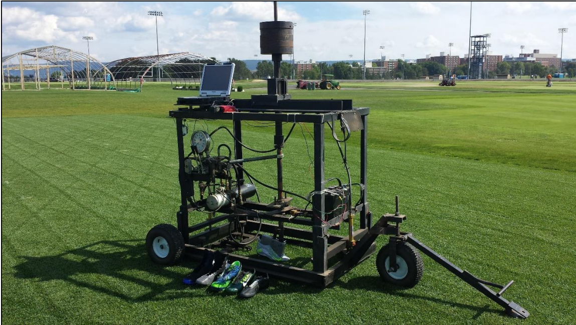
Figure 5. Pennfoot traction tester
