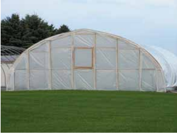
Fig. 1. Pythium chamber with plastic-covered wooden frames sealing the ends of the chamber.
