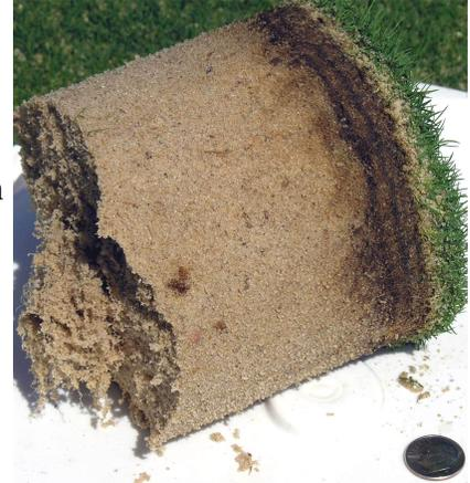
The low-flux system used pressurized ultra-pure (CO<sub>2</sub>-free) air to prevent anoxic and/or CO<sub>2</sub>-rich conditions. Except the gaseous CO<sub>2</sub> residing within pores of the plug (assumed to be equal across all cores removed from the identical green on the same day), microbial respiration comprised the sole future source of CO<sub>2</sub>
