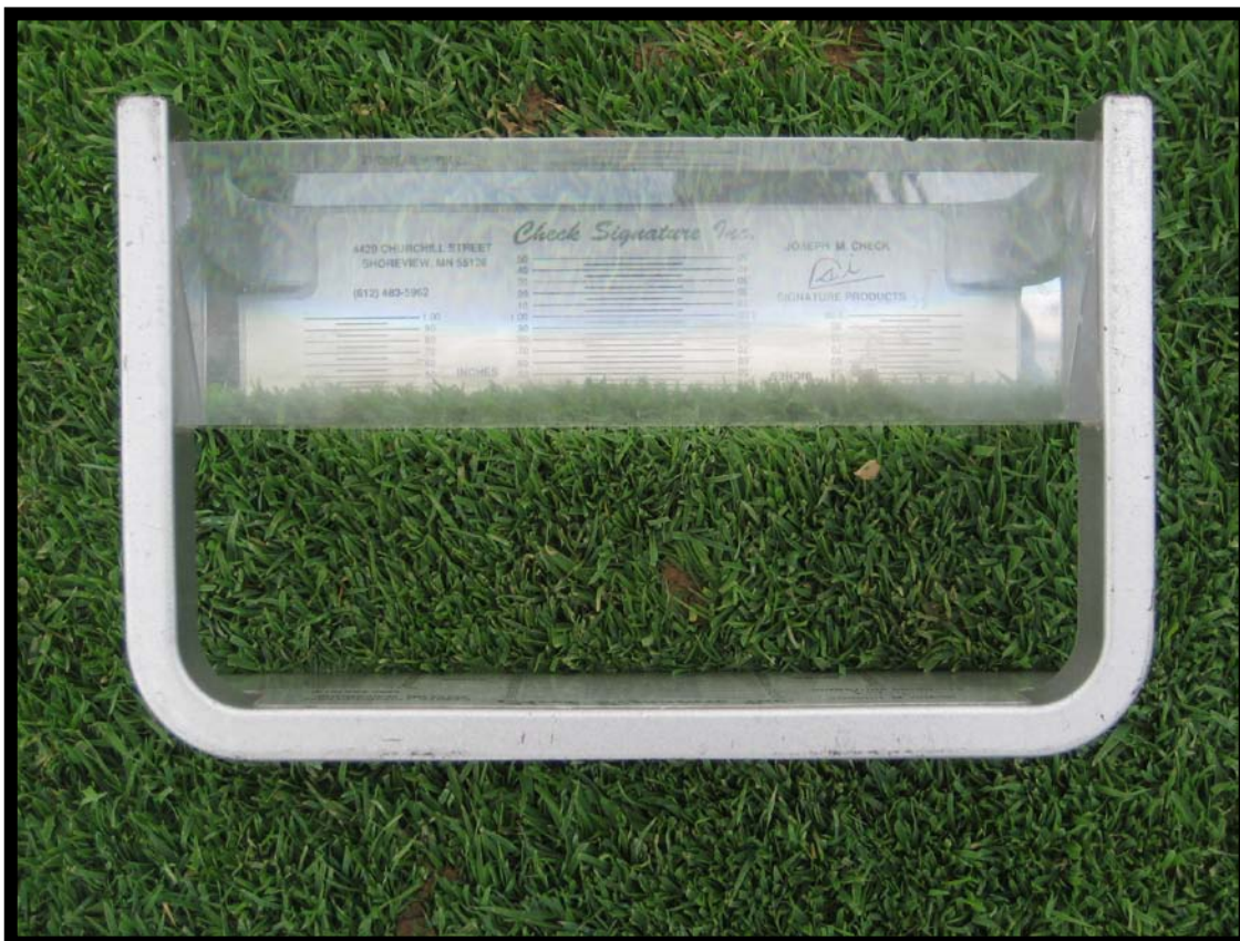
Figure 2: Creeping bentgrass heights were monitored using a Turcheck 1 Prism.
