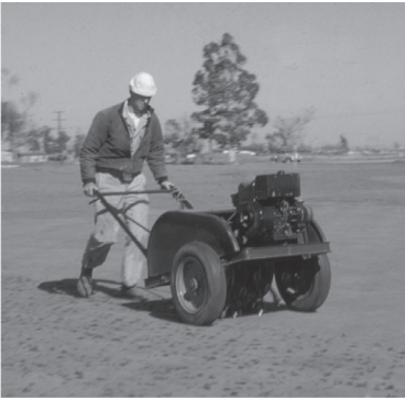
Photograph of an aerifier taken in 1947. (Photo courtesy of Jim Snow, USGA Green Section)
