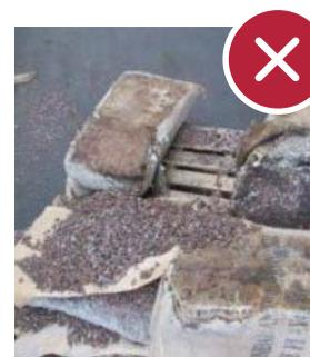
Secondary mould due to excess moisture during shipping/storage.
