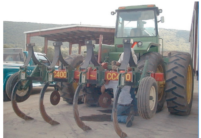
Figure 1. A sub-soiler (above) a tillage implement with few, stout, non-moving parts is recommended for initial loosening of roadside sites. Roto-tillers are more suitable for incorporating topsoil or organic matter.
